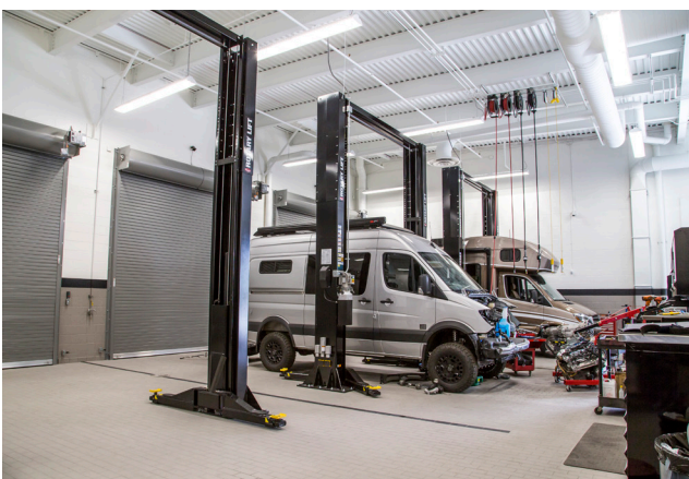
The service areas are equipped advanced technologies throughout, including standard and oversized van lifts.
