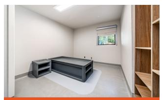
Patient areas include Mondo resilient sheet flooring with an Integral Cove Base, a rubber surface that is sound-absorbent, slip-resistant, comfortable, and easy to maintain. Installation of impact-resistant windows and ligature-resistant furniture and millwork ensures a secure and safe environment for patients.
