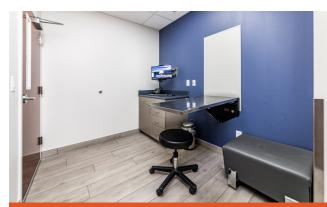
Private exam rooms are equipped with a fold down table and FRP wall panel for flexibility of use, and the porcelain plank floor tiles are aesthetically pleasing and resilient. In addition to the standard exam rooms, space inventory includes specialty feline exam, outdoor exam, and euthanasia comfort rooms.
