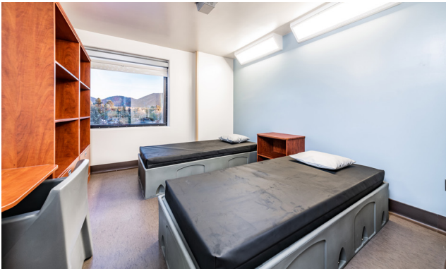
Patient rooms include ligature-resistant furniture, impact-resistant windows, and sheet flooring with a rubber surface that absorbs sound, slip-resistant, and easy for staff to maintain. These features ensure a safe and secure environment for patients.
